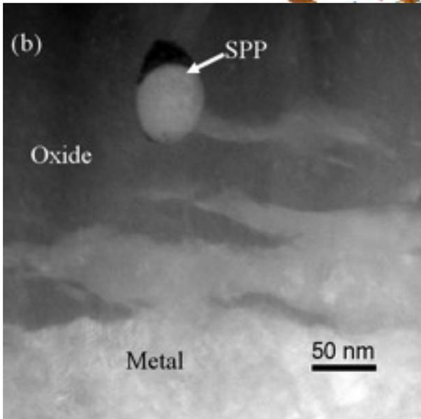
SPPs may have an important role in determining the mechanism of H pickup
