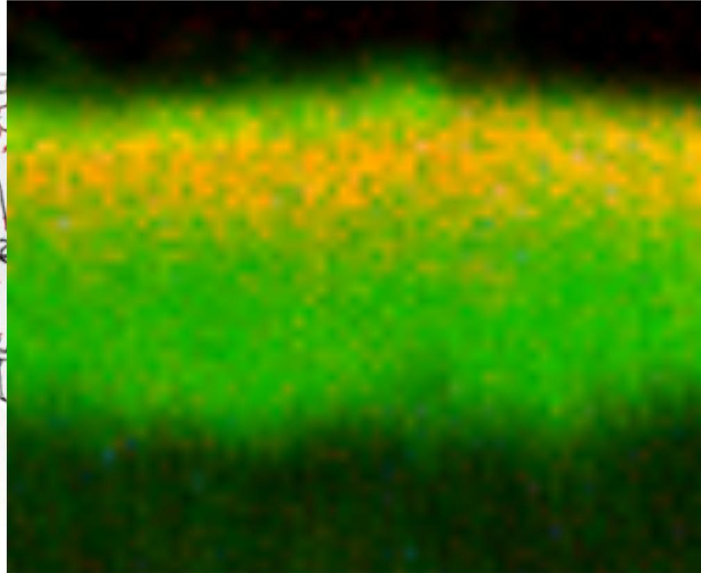
$^{18}\text{O}$  can only diffuse into oxide along monoclinic  $\text{ZrO}_2$  grain boundaries
