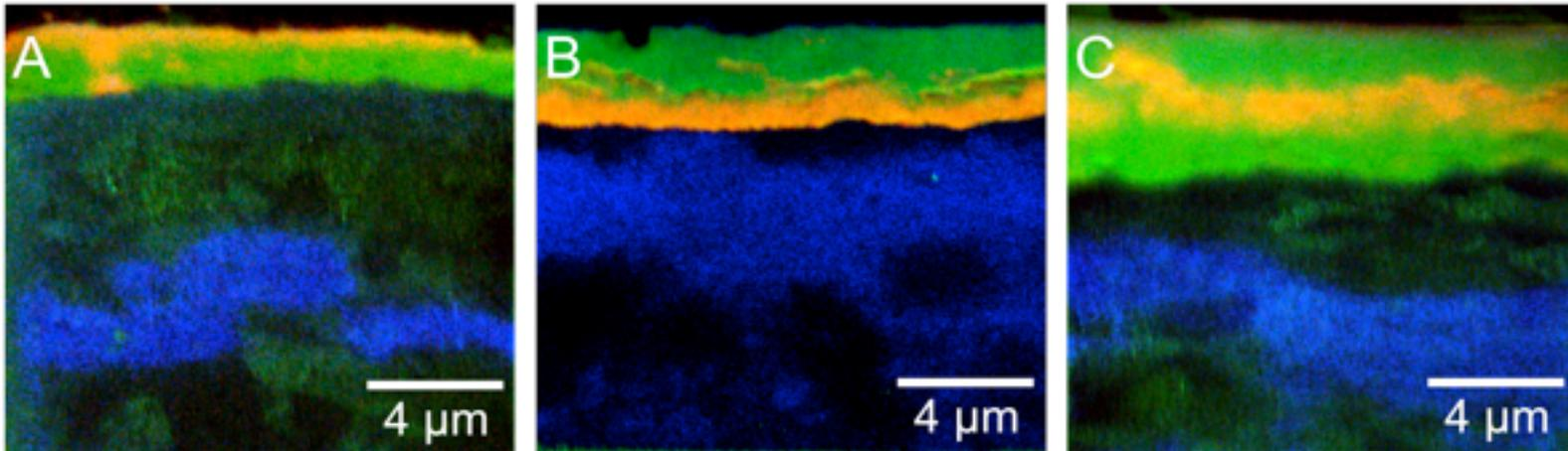
Figure 6: Colour merge images showing the relative locations of the  $^{18}\text{O}^-$  (red),  $^{16}\text{O}^-$  (blue) and  $^2\text{H}^-$  (green) signals. Hydrides are found below the metal/oxide interface but no deuterium was detected in the oxide layer. A: 34 + 20 day sample, B: 80 + 20 day sample, C: 160 + 20 day sample.
