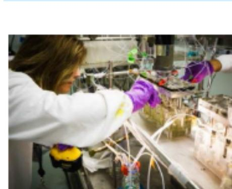
Platform of mixers and settlers to validate the performance of the selective uranium extraction process on a laboratory scale
