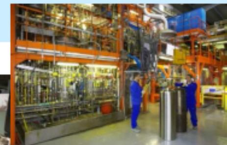
General view of the evolving vitrification prototype equipped with a cold crucible melter adapted for nuclear environments at Marcoule
