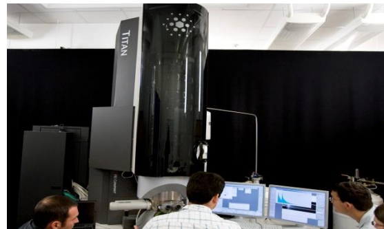
Ultra-high resolution TITAN microscope
