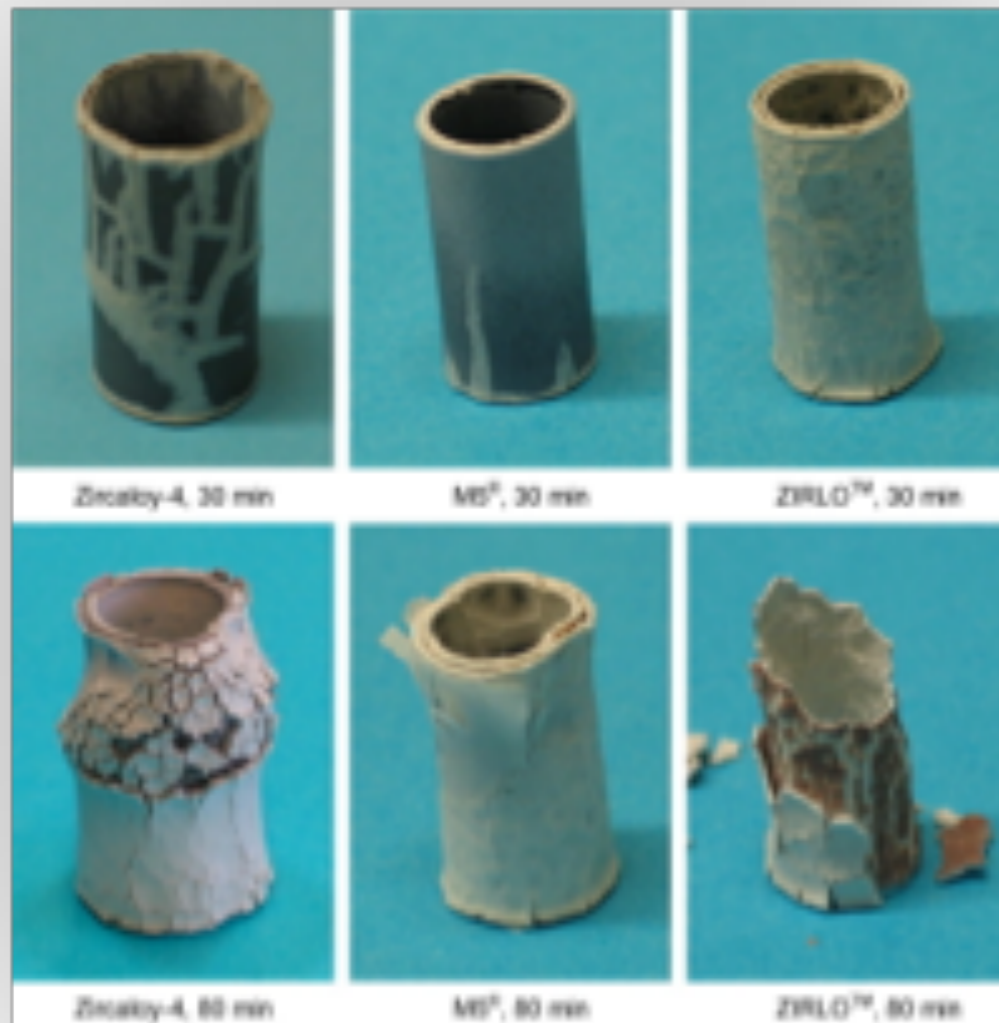
Hi T steam tests on zircalloys [Y. Lee (KAIST)]
