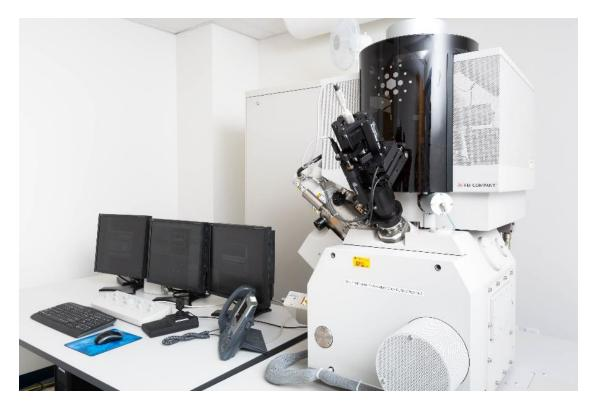
FEI HELIOS NANOLAB 600 Dual Beam FIB/SEM
