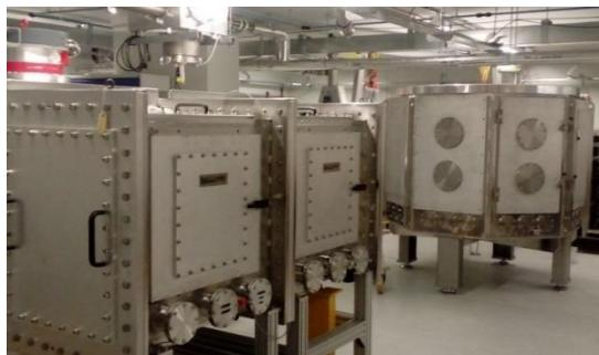
Compact GeV electron accelerator and gamma-ray source
