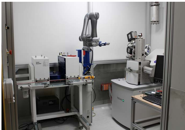
Inside a shielded research room (GBq), showing robotic loading for the SEM.
