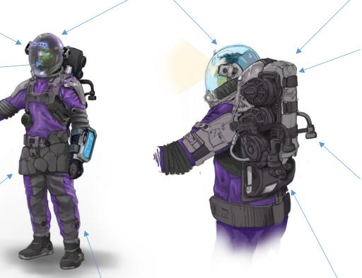
Back-mounted unit includes SCBA, Ekso augmented strength suit, power supply and suit cooling system.
