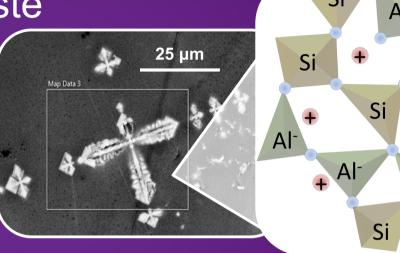
Geopolymers for Intermediate Level Waste (alternative to cementitious grout)
